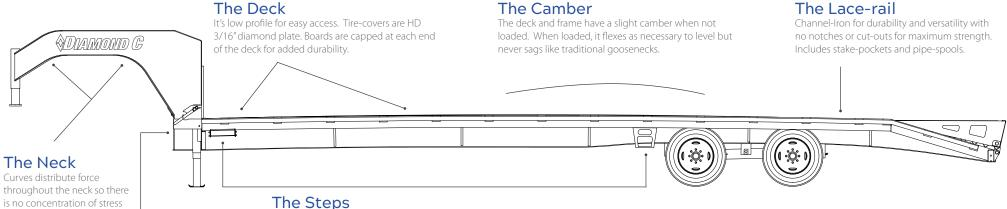
The retractable front deck steps solve the common issue of traditional front deck steps being bent in low clearance situations.
